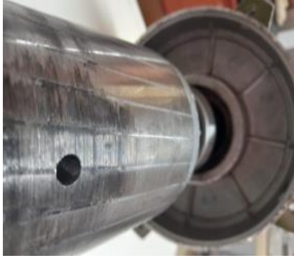
Figure 4. Induction motor rotor bar fracture (broken)
