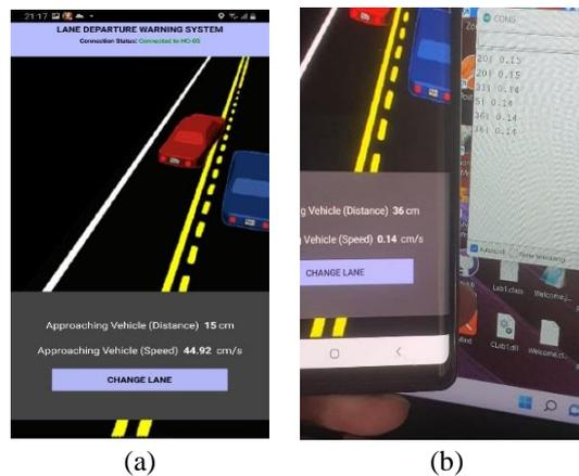
Figure 7. Distance and speed data received from approaching vehicle (decision aid) (a) application and (b) terminal
