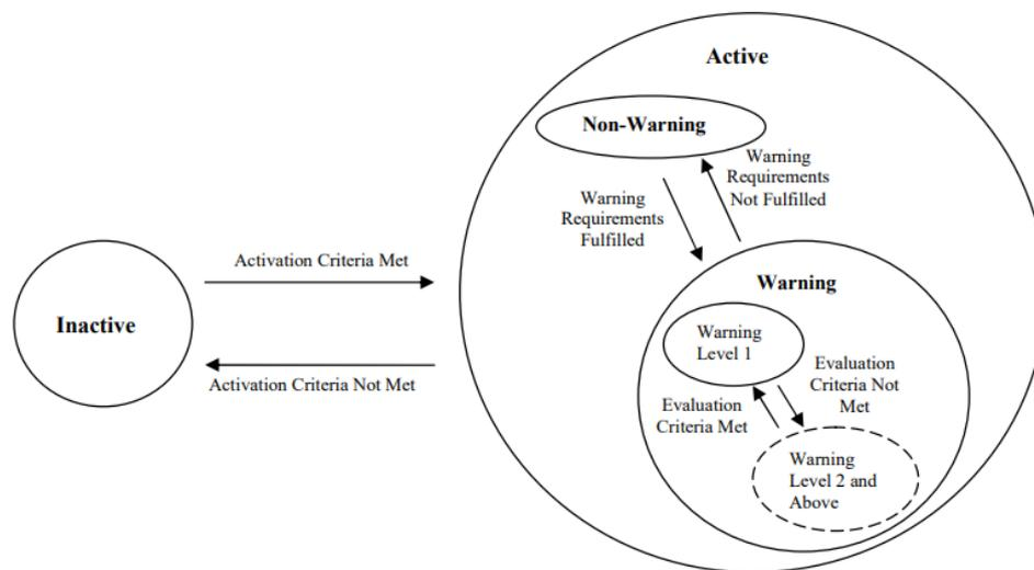
Figure 1. ISO 17387:2008 state diagram for LCDAS
