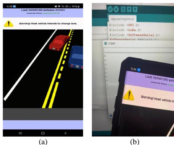
Figure 8. Alert message received from host vehicle (warning) (a) application and (b) terminal
