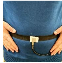
Figure 8. The fabricated antenna under test
