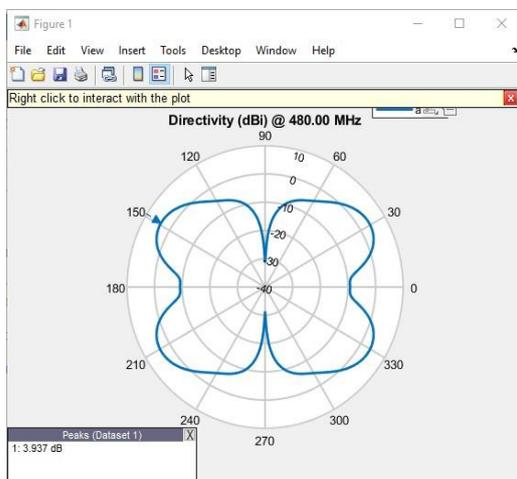
Figure 14. E-plane radiation pattern of batch 2
