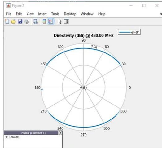
Figure 5. H-plane radiation pattern of batch 1
