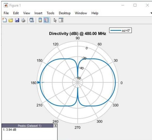
Figure 4. E-plane radiation pattern of batch 1
