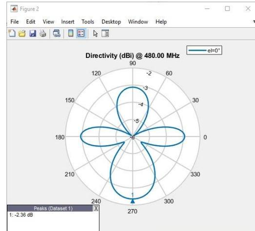
Figure 17. H-plane radiation pattern of batch 2
