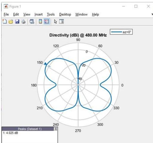
Figure 6. E-plane radiation pattern of batch 1
