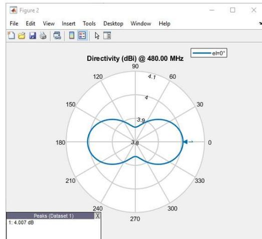
Figure 13. H-plane radiation pattern of batch 2
