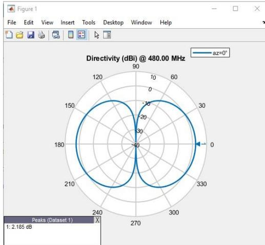
Figure 10. E-plane radiation pattern of batch 2
