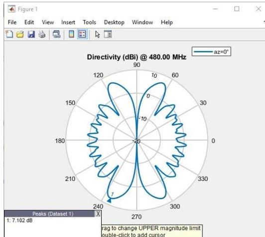
Figure 16. E-plane radiation pattern of batch 2
