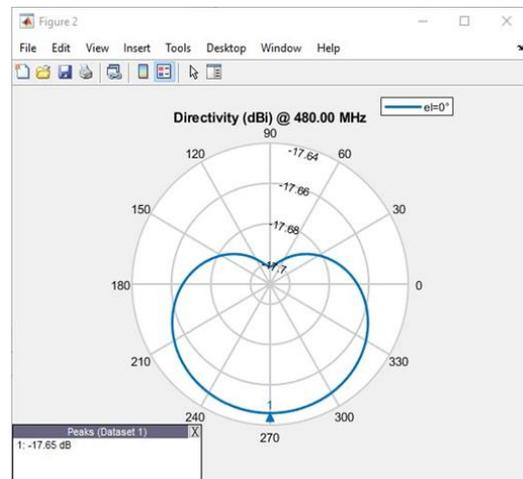
Figure 7. H-plane radiation pattern of batch 1
