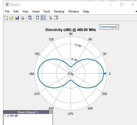
Figure 11. H-plane radiation pattern of batch 2
