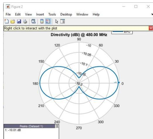
Figure 9. H-plane radiation pattern of batch 1
