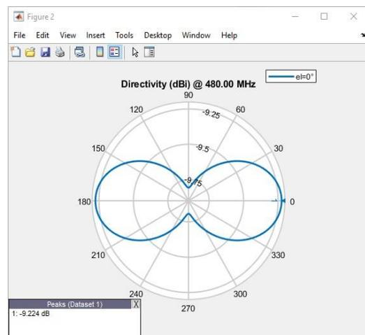
Figure 15. H-plane radiation pattern of batch 2
