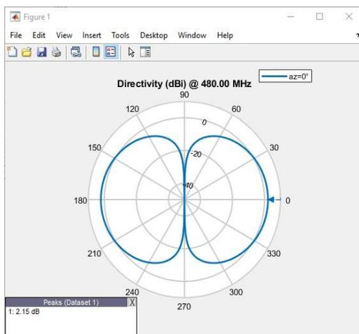
Figure 2. E-plane radiation pattern of batch 1
