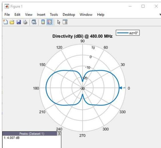
Figure 12. E-plane radiation pattern of batch 2
