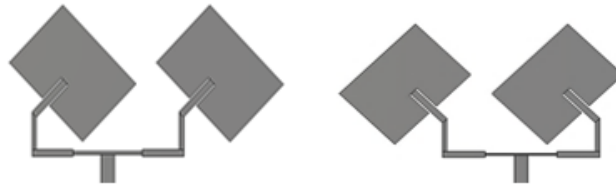
Figure 3. 1x2 array with + 45° and 1x2 array with -45° polarization angles
