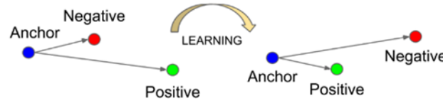
Figure 2. Triplet loss minimizes the distance between anchor and positive (both have the same identity information) and maximizes the distance between anchor and negative (both have different identity information) [11]
