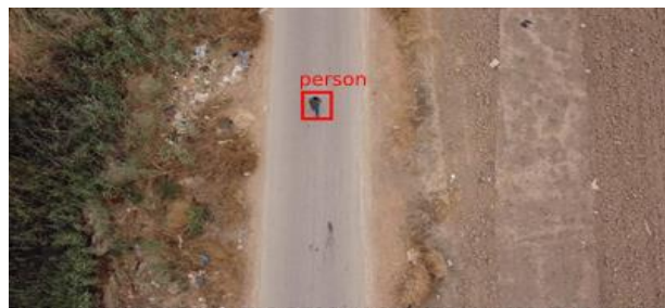
Figure 7. A drone is able to detect person from high distance using YOLO
