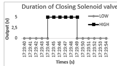
Figure 14. Duration of closing solenoid valve action
