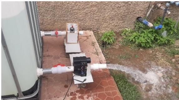
Figure 11. Real test of opening solenoid valve
