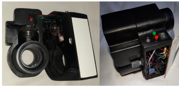
Figure 10. The final solenoid-valve realized on assembled and dismantled mode
