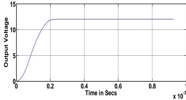
Figure 4. Output voltage of robust reaching law
