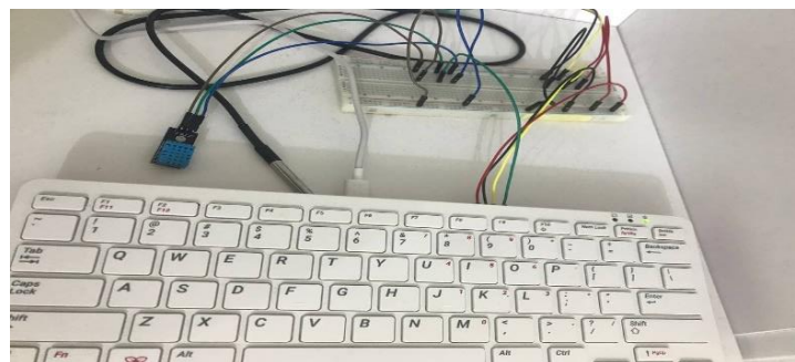
Figure 4. Raspberry Pi 400 with waterproof sensor and temperature-humidity sensor
