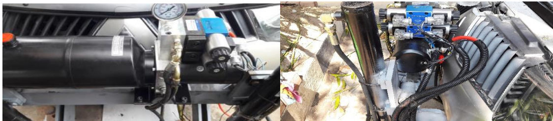
Figure 7. Installed hydraulic pump at the front of vehicle
