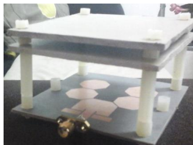
Figure 7. The prototype of the OMYA with double DPS layer
