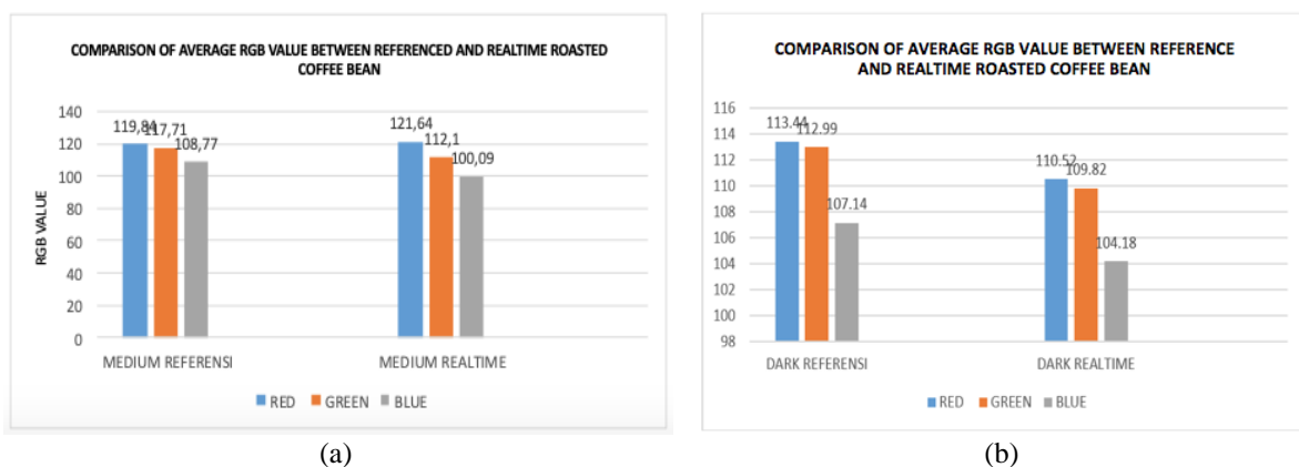
Figure 7. Comparison of average RGB value at, (a) medium level, (b) dark level
