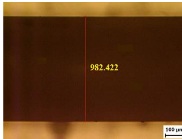
Figure 3. Etching side view measurement of fiber sensor probe for etching time=2 s
