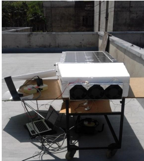
Figure 1. Outdoor experimental of photovoltaic thermal solar air collector
