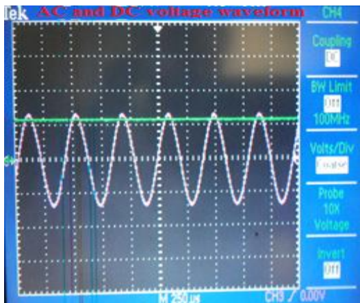
Figure 9. AC voltage waveform of receiver coil and DC voltage output of rectifier circuit
