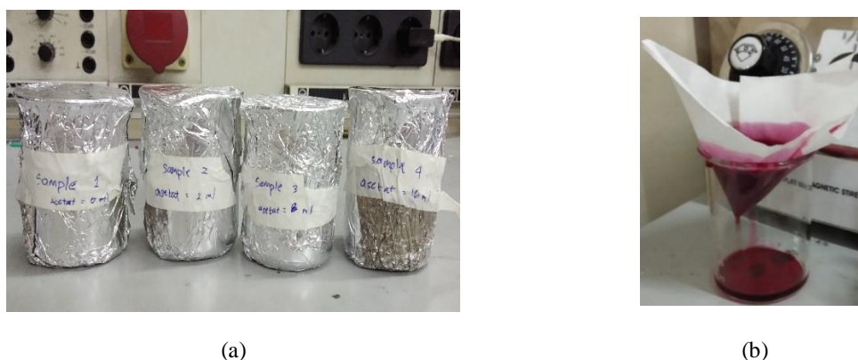
Figure 2. (a) Dye soaking with different amount of acetic acids, (b) Dye filtering
