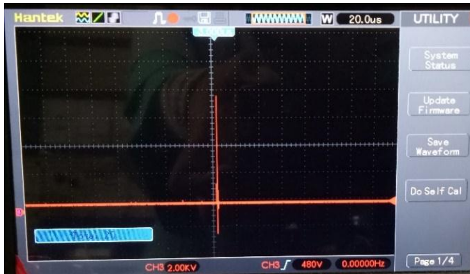
Figure 7. Output voltage with no load ( R=1\text{ M}\Omega\ 1\text{W} )
