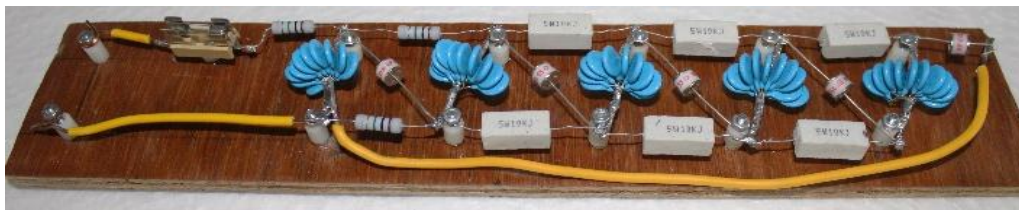
Figure 3. Realization of a 4-stage Marx generator with GDT
