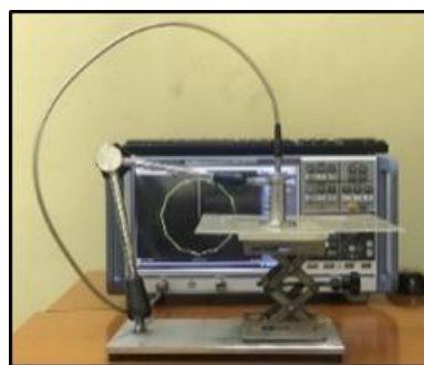
Figure 3. The open-ended coaxial probe for the determination of dielectric properties of PLA substrate
