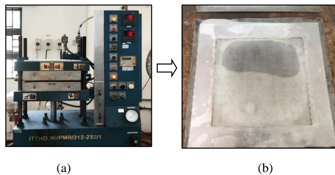
Figure 2. Fabrication process of PLA substrate, (a) Hot press machine, (b) PLA substrate
