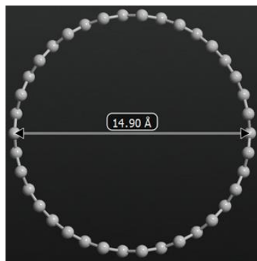
Figure 4. Diameter of (19, 0) CNT
