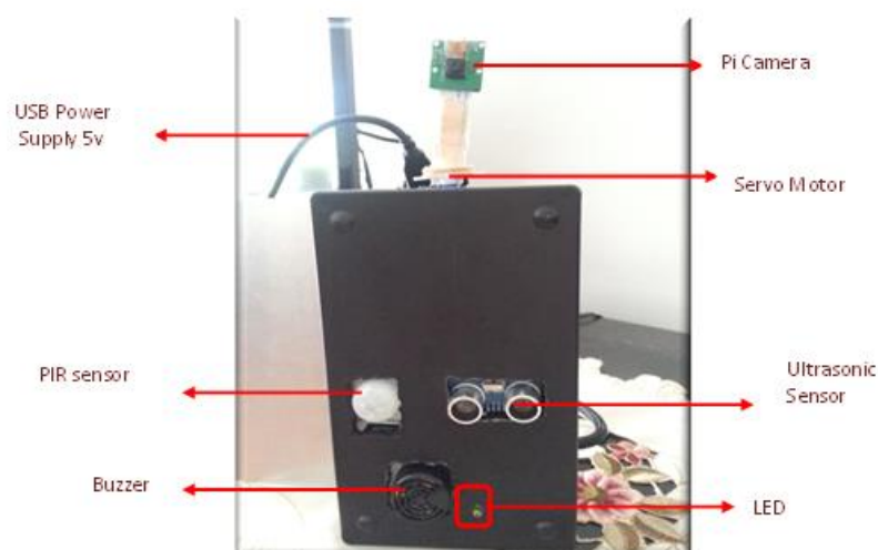
Figure 5. The complete setup of the surveillance system
