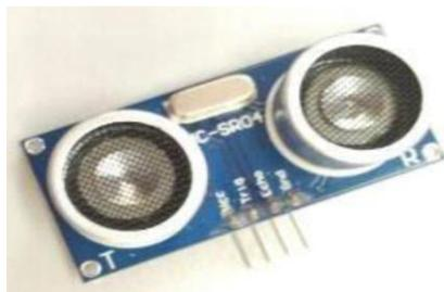
Figure 1. Ultrasonic sensor
