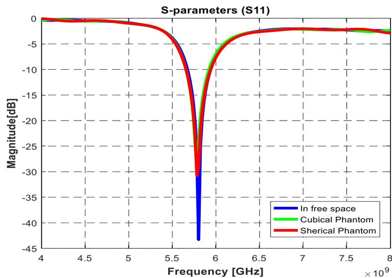
Figure 4. Comparison of the simulated reflection coefficient of the designed square ring antenna in free spaces and human head
