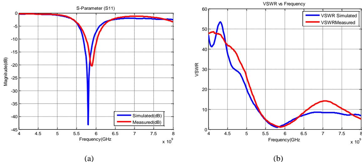
Figure 3. Comparison simulated and measured results of proposed antenna in free space (a) S11 and (b) VSWR
