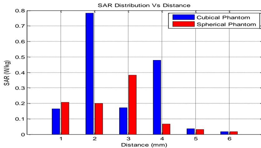
Figure 6. Comparison of SAR variation against distance between human head and antenna
