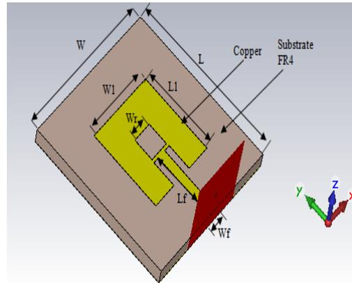
Figure 1. Top view of printed antenna
