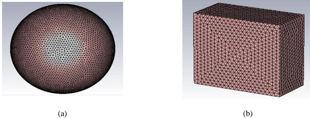
Figure 2. Proposed phantom models of human head (a) spherical phantom (b) cubical phantom
